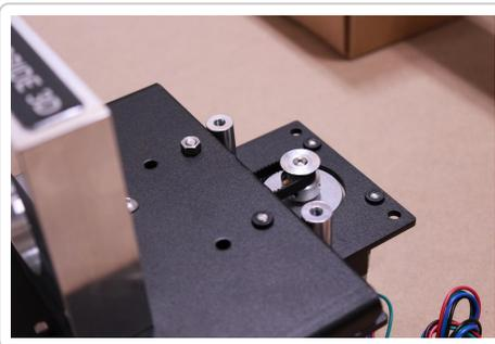
Ensure that you have only finger-tightened the Idler Assembly before tightening the Tensioning Screw.
