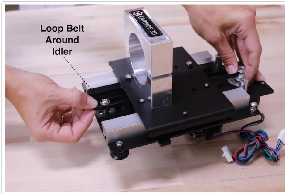
The Idler can move up and down in its groove. You may have to loosen the nut to move the Idler.
