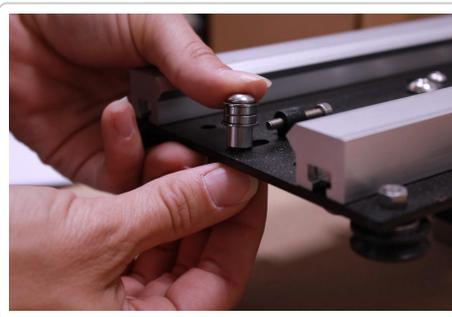
Carefully remove the nut while ensuring the remaining components stay on the bolt. Insert the bolt through the slot located at the bottom of the plate - shown in the image below. Secure in place by finger-tightening the nut on the opposite side of the X Carriage.
