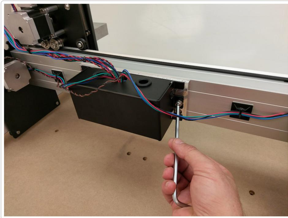
After your wires have been connected to the correct ports, install the enclosure cover using the included M6 x 8mm Socket Head Cap Screws (one on each side).
