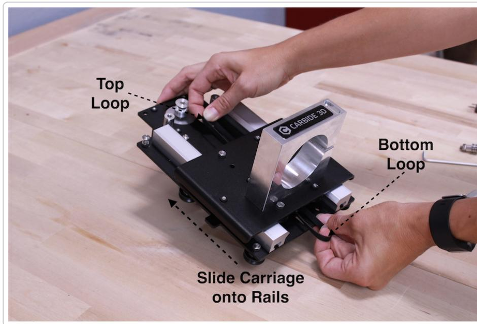
Align the Z-carriage with the bottom of the X-carriage, making sure the eccentrics on the Z-carriage are positioned on the left side, as shown in the image below.
