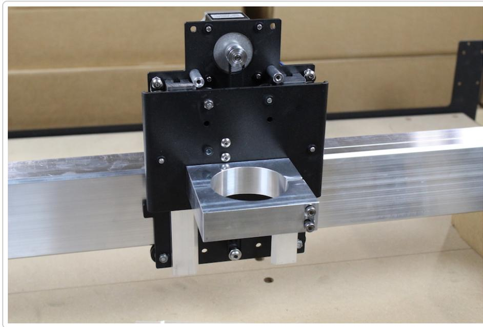
Slide the X/Z Carriage on the rail from the right hand side. Because the V-wheels will be as loose as they can, the carriage will slide easily down the rail — be careful not to tip the rail too high causing the carriage to slam into the left Y plate.
