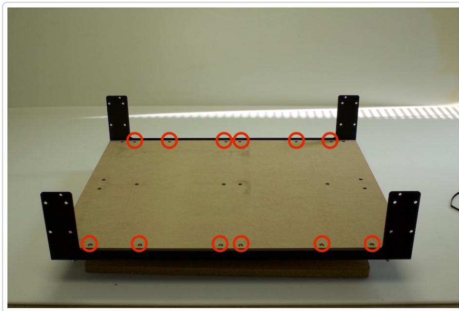
Using the hardware found in the package labeled 'WASTEBOARD', assemble the base frame of the machine.
