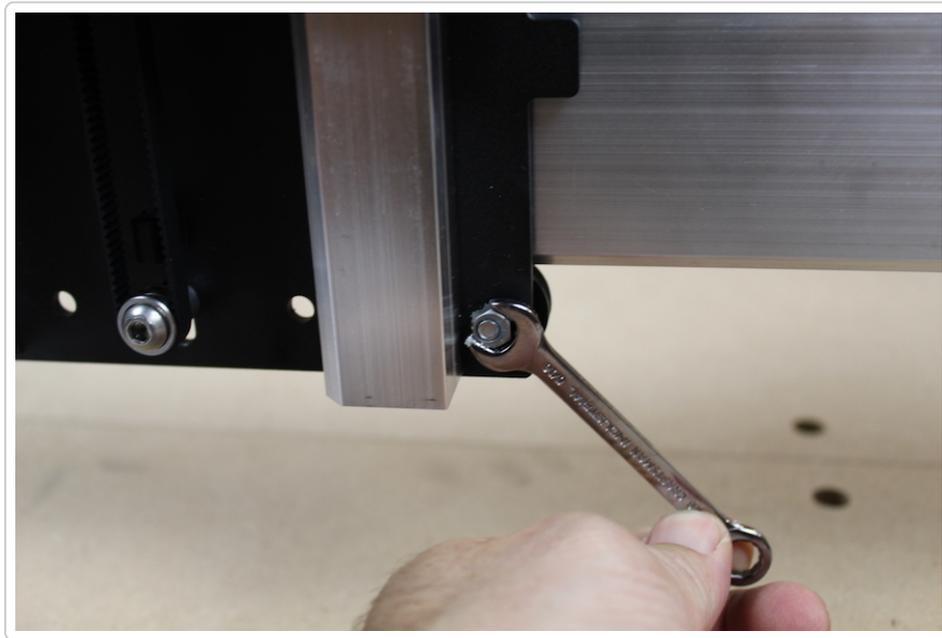
You do not need much tension in order for the carriage to be secure. The wheels should only be snug against the rail.
