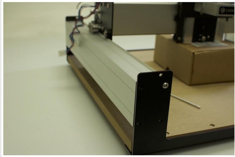
After the front is finished, move around to the back of the machine and install all 4 screws on each side of the gantry. Again, these screws should not be fully tightened. We will do that in the 'squaring your machine' section.
