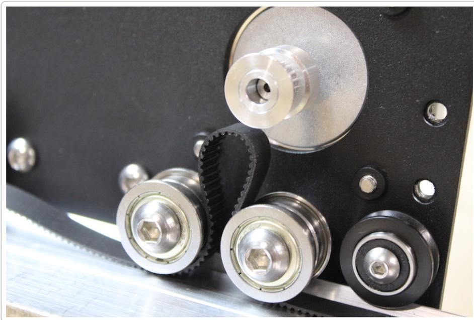
Using another M5x10mm screw, tension the belt clip against the front of the machine.
