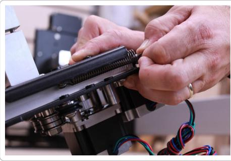
Turn the X/Z Carriage on its other side and attach second spring in identical manner as shown in the image below.
