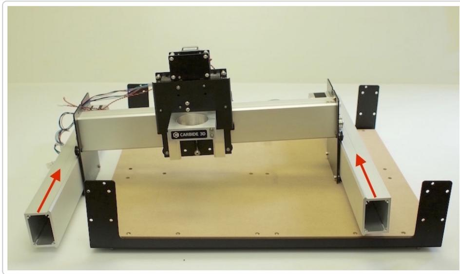
Using the box as a support, position the gantry system into the base frame. You may need to loosen the base frame assembly if there is not enough clearance to insert the rails. Slide the gantry system in from the side. If you have two people, you can also set it in from the top.
