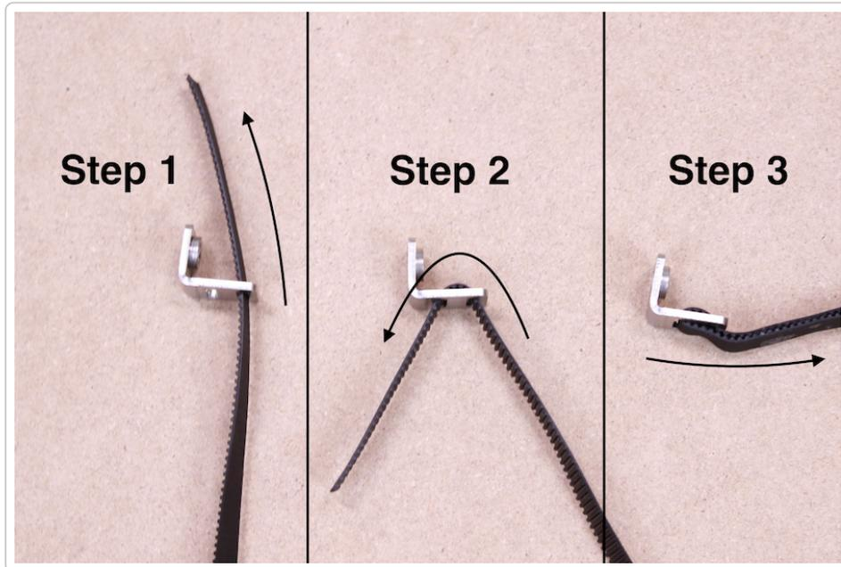
The proper routing is: Up from the bottom, Down through the top, Back towards the front. Pull about 2" of
