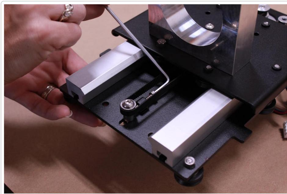
Use the hex wrench to tighten the Tensioning Screw as shown in the image below. As the Tensioning Screw is tightened, it will push on the Idler Assembly.
