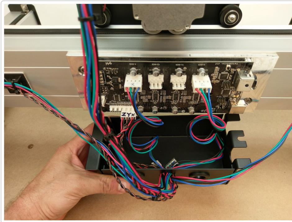
Attach the X and Z axis stepper motors to their respective ports (labeled on the silkscreen as well).
