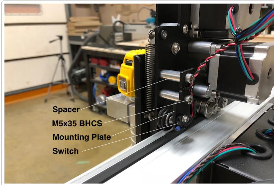
Slide the screws through the X-axis plate, attach spacers, then attach entire assembly to the back of the X-axis plate, using the built in nuts.
