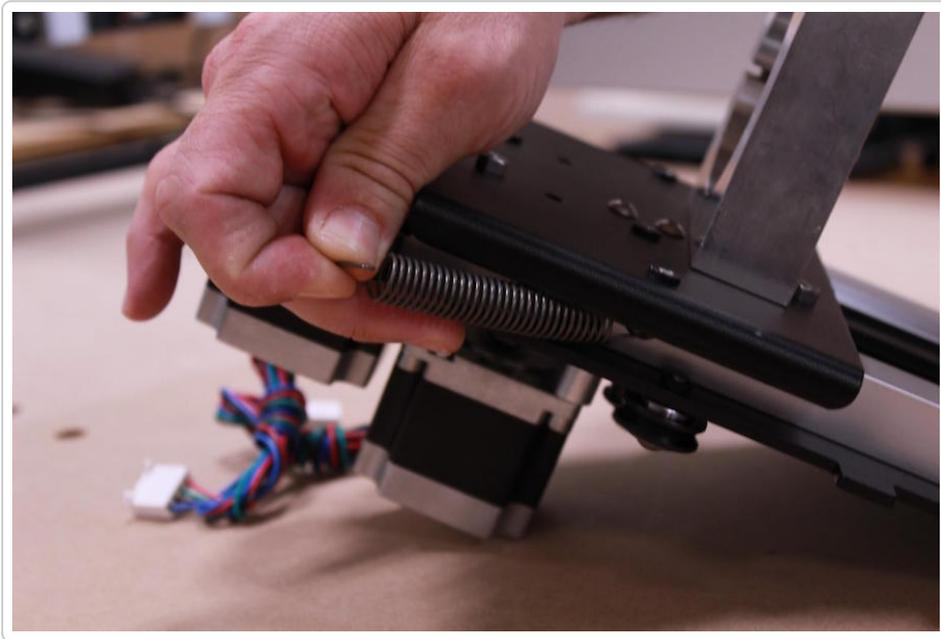
Using the 2x M5x55mm screws, install into spindle mount. Do not tighten at this point, we will secure these screws after we install the spindle later in this guide.
