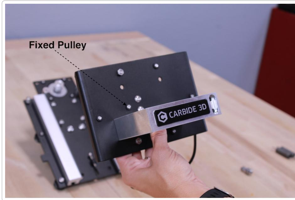
Align the spindle mount with the bottom set of through holes on the z-carriage. The Carbide 3D logo should go right side up, but the position of the pocketed hole on the spindle mount does not matter (left or right is fine).
