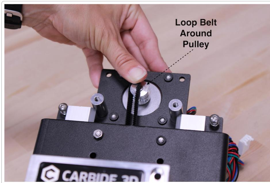
**NOTE:** If you had to loosen the Idler nut to move it, move the Idler down to provide some tension on the
